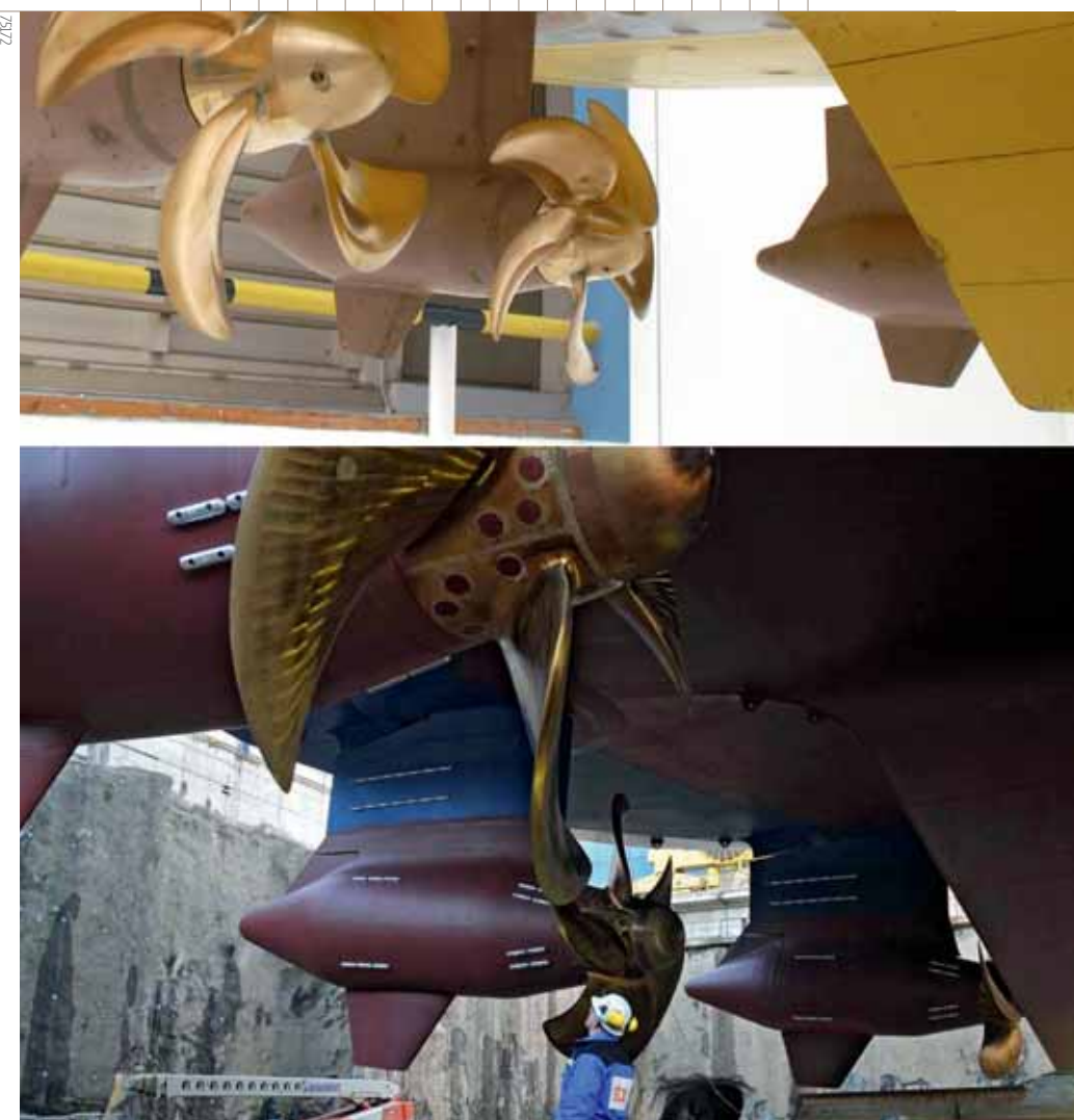
Full and model scale pods (model scale image is mirrored)
