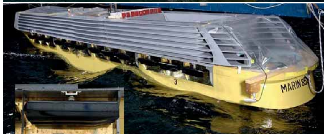
Model tested in severe weather conditions. Lifeboats mounted on force transducers.
