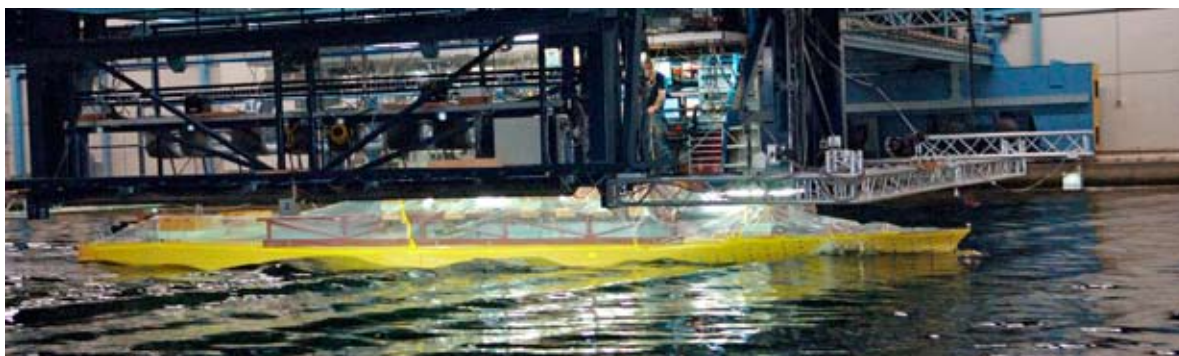
12 m free-sailing model with 70 pressure gauges
