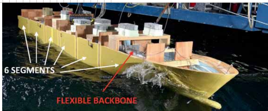
6-segmented model mounted on a flexible backbone.
